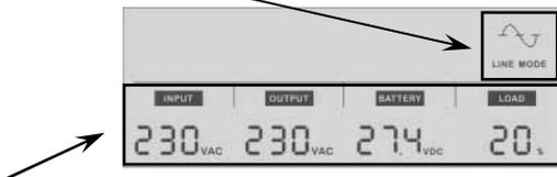
The bottom half of the display shows in the INPUT and OUTPUT voltages of the UPS, the battery (charging) voltage (BATTERY) and the percentage capacity utilisation (LOAD) of the UPS.
